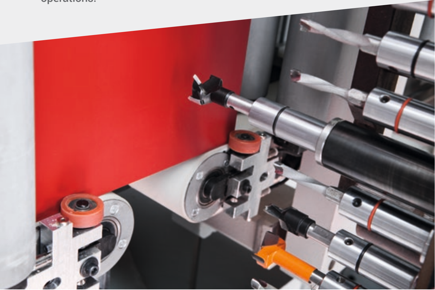
The longer-stemmed spindles allow users to successfully perform all drilling operations, guaranteeing optimum quality standards.
