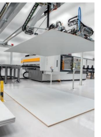
The Winstore automated magazine stacks sheets of different sizes and materials, including mixed ones, with no need for operator intervention. The reorganisation of sheet magazine and stacking can be carried out automatically, out of working hours.
